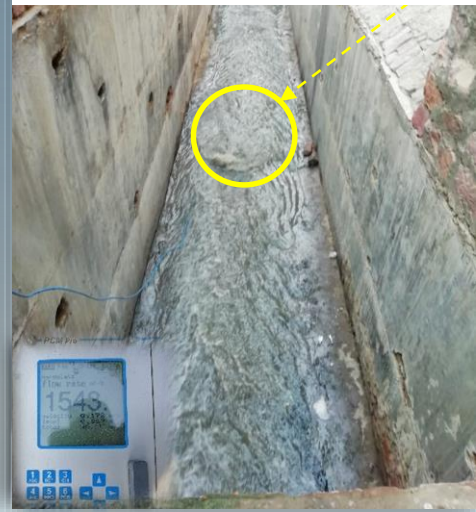
Channel Shape: Rectangular; Channel Dimension: 1900 mm (w) x 1500 mm (H)
